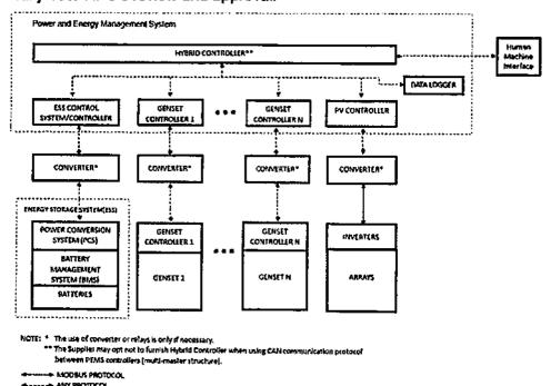
Figure 1: PEMS and Communication Diagram
